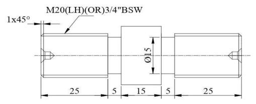
2. Prepare the specimen and make the Eccentric turning as shown in figure using the Lathe.
