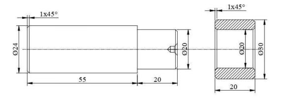
1. Prepare the specimen and make the Step turning & BSW and Metric Threadcutting as shown in figure using the Lathe.
