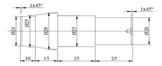
2. Prepare the specimen and make the Step turning & Knurling as shown in figure using the Lathe.
