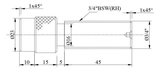
4. Prepare the specimen and make the Shaft and Bush as shown in figure using theLathe.
